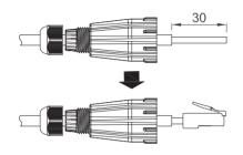
Step 2: Plug in the modular plug with socket, turn tight the boot then completed the mating.
